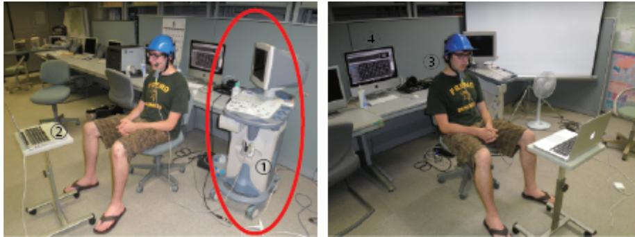
Fig. 1: Recording Environment. 1. Ultrasound camera, 2. Corpus is shown on a display, 3. Combination of helmets and transducer, 4. iMac for recording ultrasound movies.
