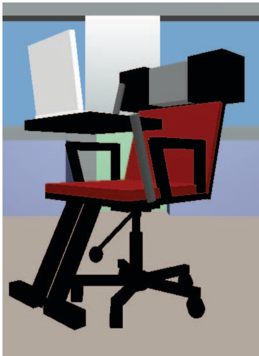
Figure 2: For its haptic output modality, servomotors render kinesthetic force display, rotating each S h air e under networked control. Note the nearphones straddling the headrest.
