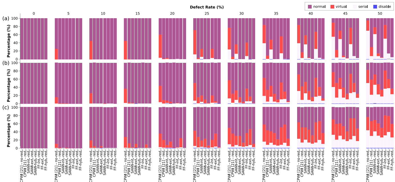
Fig. 9: Defect-rate evaluation with random defect distributions (injected to redundant TSVs): (a) Layer size: 2 \times 2 (4 routers, 16 TSV clusters); (b) Layer size: 4 \times 4 (16 routers, 64 TSV clusters); (c) Layer size: 8 \times 8 (64 routers, 256 TSV clusters) .
