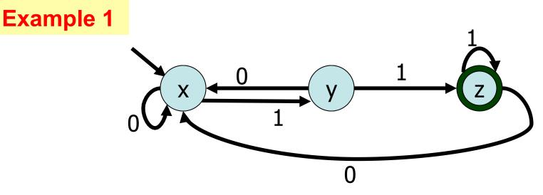
The DFA above can be simulated by the grammar  $x \rightarrow 0x \mid 1y$   $y \rightarrow 0x \mid 1z$  $z \rightarrow 0x \mid 1z \mid \lambda$
