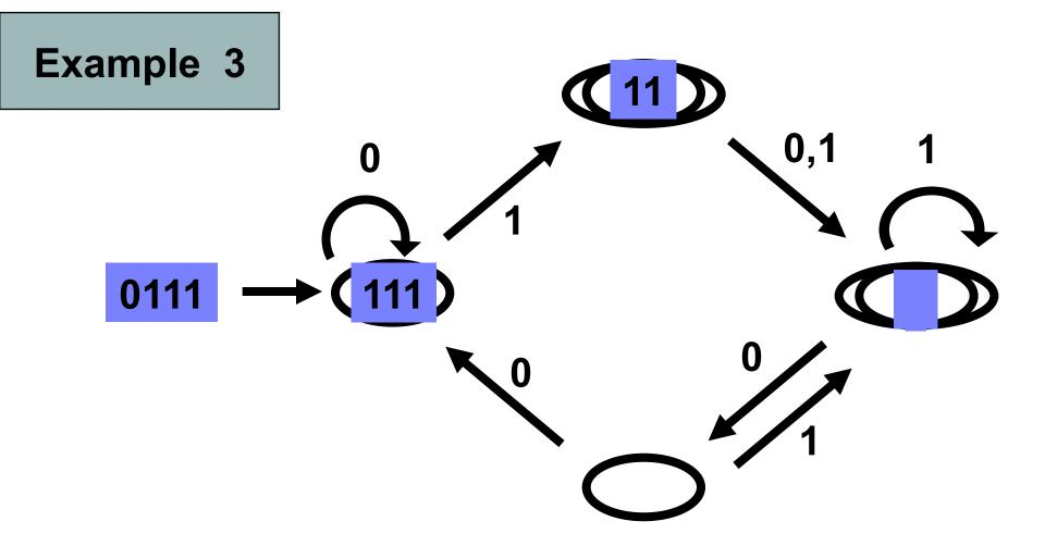
The machine accepts a string if the process ends in a *final state*
