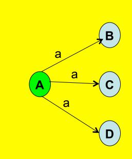
From ONE state machine can go to MANY states on one input
